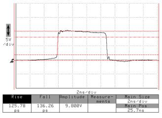
The AVMP series of pulse generators offer 10V or 20V outputs with sub-nanosecond rise times, and pulse widths variable from several nanoseconds up to 100 ns, 1 us, or 10 us.
